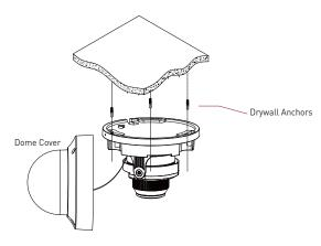
4. Fix the dome cover back onto the mounting base by installing the three dome cover screws into the camera and tightening it once the position is secured.
